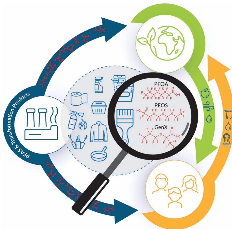
Figure 1. Schematic showing the cycle of PFAS. PFAS are synthesized for incorporation into commercially available products. Contaminated soils, groundwater, and waste from industry production and use and human use of PFAS-containing products impact human and environmental health. Humans release PFAS into the environment through waste and wastewater, where the chemicals accumulate. In turn, the accumulation of PFAS from industry and waste causes exposure through contaminated sites (including sites contaminated with Aqueous Film-Forming Foam (AFFF)), air pollution, water pollution, and contaminated food.
